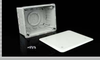
Material:PC ABS, self snuffing, halogen-freeDimension:box 196 x 156 x 85 up to 140 mmcover 210 x 170 mm
