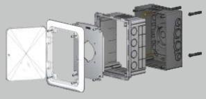
Set of **KUZ-VI** is suitable for installation in thermal insulation systems. The box is the same like KUZ-V and complete with supporting tube, inside and outside insulation, set of accessories for mounting the tube on the wall and also screws for mounting the box on the tube.
