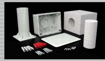
Material: Dimension: PC ABS, self snuffing, halogen-free box 196 x 156 x 85 up to 140 mm cover 210 x 170 mm Variant **KUZ-VO** is conceptually the same like KUZ-V, only instead cover V 180 is set with cover VO 180, opening the cover is without using any tool.
